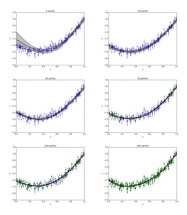
Figure 53: Gaussian process fit to noisy measurements of a quadratic, for different sizes of training set, as stated in the title of each panel.
