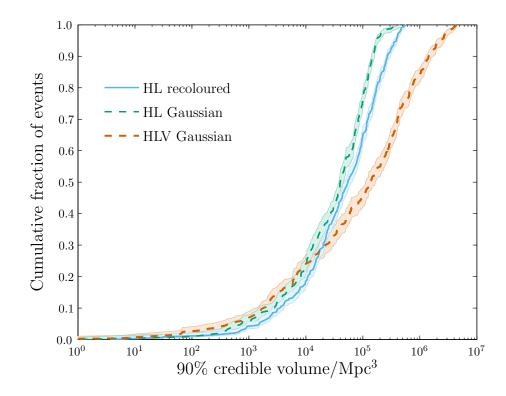
Figure 64: Cumulative distribution function of 90% credible volumes for events observed by the ground-based detector network. The credible volumes were computed by fitting a Dirichlet Process Gaussian Mixture Model to posterior samples generated by LALInference. Figure reproduced from Del Pozzo et al. (2018).
