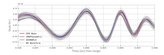
Figure 57: Comparison of several approximate waveform models to random draws from a Gaussian process interpolant trained on numerical relativity simulations. Reproduced from Williams et al. (2020).
