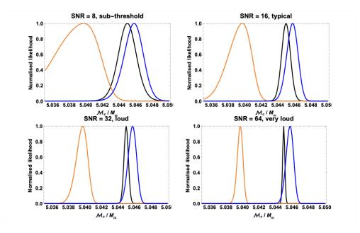
Figure 56: Comparison between uncorrected, corrected and "true" likelihood for inference with waveform models that include model error. The corrected likelihood uses a Gaussian process to model the waveform error and then marginalises this out of the likelihood. Reproduced from Moore et al. (2015).
