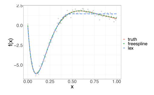
Figure 62: Nonparametric regression fit to noisy measurements of the function  $f(x) = 26 \exp(-3.25x) - 4 \exp(-6.5x) + 3 \exp(-9.75x)$  using the freespline algorithm with a Dirichlet process prior on the probability density determining the knot locations. Figure reproduced from Edwards & Gair (2020).
